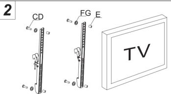
Using Long bolt(CorD), washer(ForG) and Spacer (E) to mount TV set to the aluminum siding .
