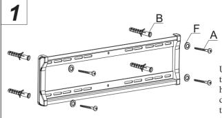
Using the bubble level to ensure the wall plate is level, Pre-drill 4 holes with a 10mm bit to 50mm deep.Insert wall anchors into the holes,then using long bolts to mount the wall to studs.
